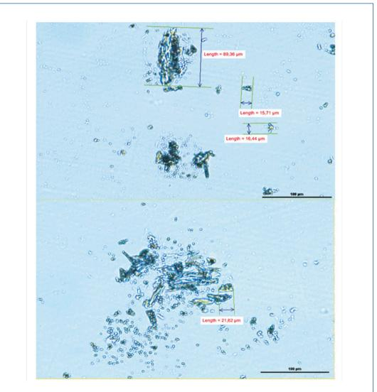
Fig. 6. View of contaminant particles in a hydraulic oil sample taken after 2 500 of use (magnification ratio:  $20 \times 10$ )
