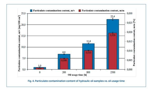
The particulate contamination content by mass increased tenfold for the first 800 h and twentyfold for the 2 500 h of the oil usage time in comparison with that of the fresh oil. The particle size distribution also changes with the oil usage time (Table 2).
