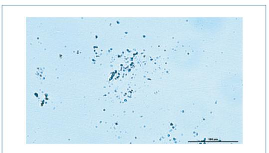
Fig. 7. View of fine-dispersed contaminant particles in a hydraulic oil sample (magnification ratio: 20×10)
